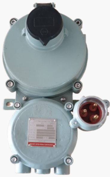
FLP Built in Transformer Gas Group IIC, IP-66, T6 Rating: 16A 24V AC
